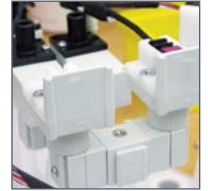
Installed assembly flexadapter with two points of test
