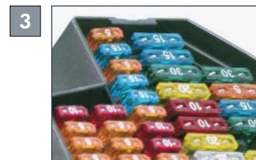
3 visual test of fuses and their positions
