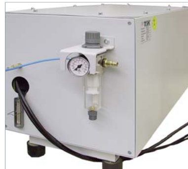
Back side: Air supply and digital I/O interface
