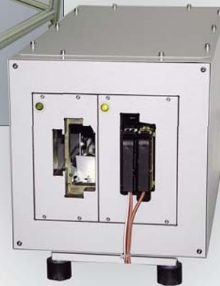
Example: VS30 as add-on system, with two test device intakes
