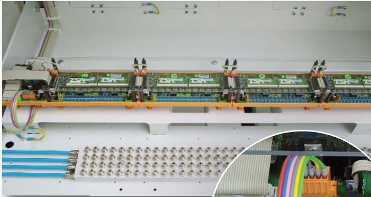
TS1500 CT, test point boards and pneumatic connections
