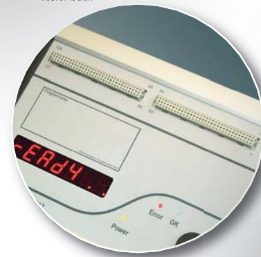
Test point interface 2 x 64pol.
